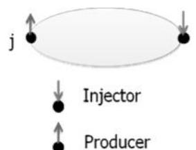
**Figure 1.** A control volume including one injector/producer pair
